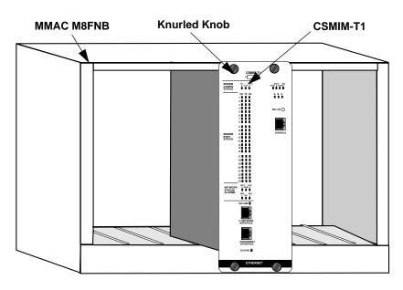
Figure 2-3 Installing the CSMIM-T1
